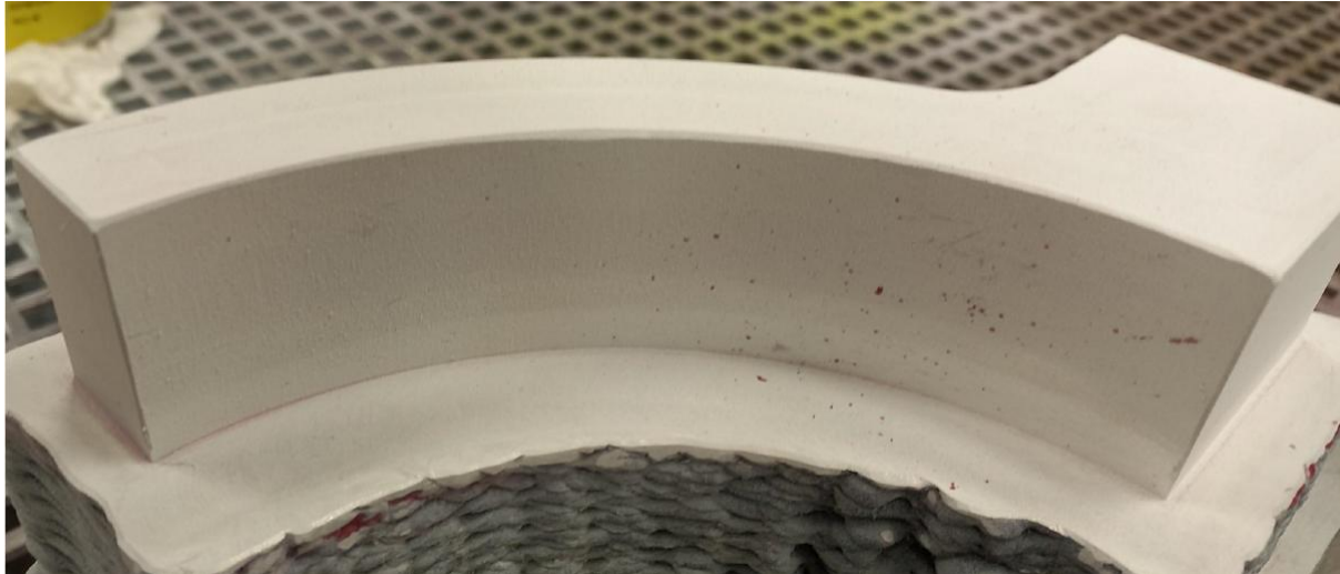
Figure 7: image of penetrant testing with round and more linear indications on a machined surface
